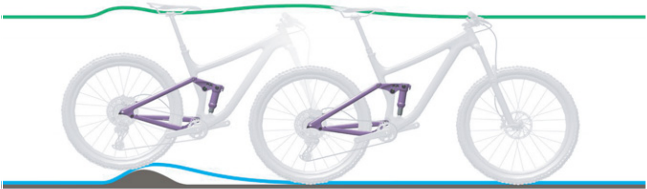
Figure 225: Excessively hard damping in the rear frame damper on bumps
