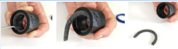
Figure 195: Removing the felt ring
