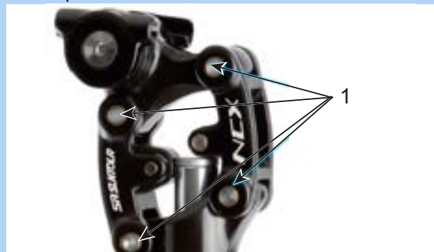
Figure 148: SR Suntour suspension seat post lubrication points
