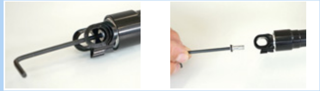
Figure 165: Unscrewing the valve cap
