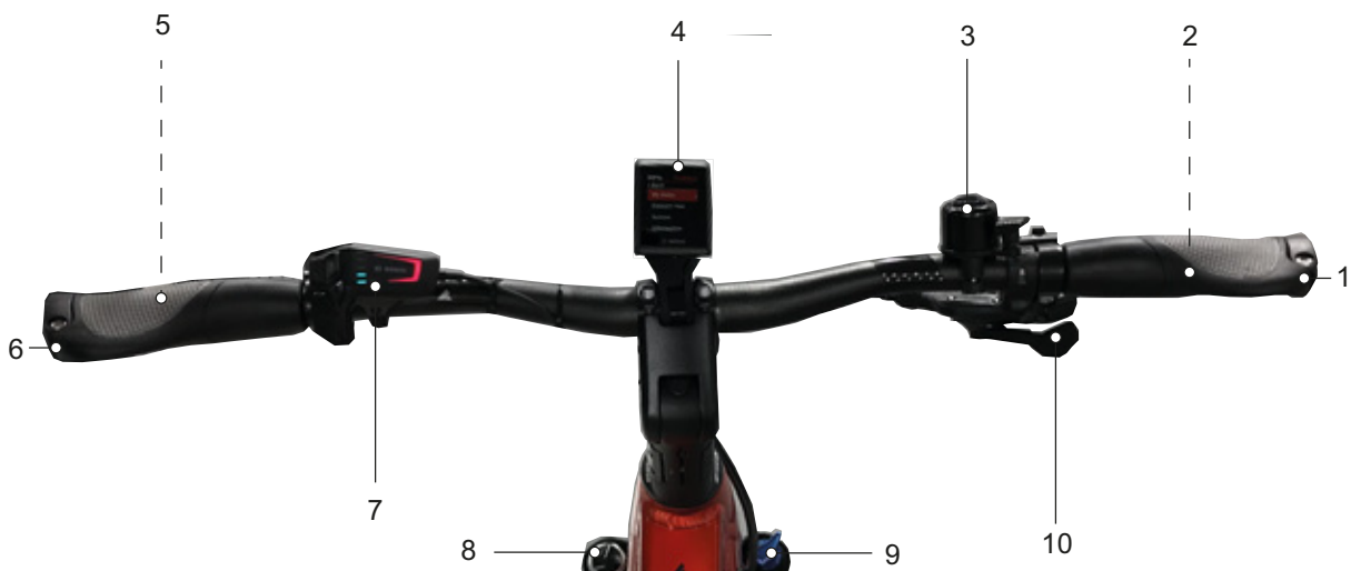
Figure 39: Detailed view of handlebars with BOSCH Kiox300, example
