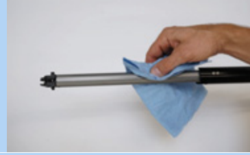
Figure 202: Cleaning the longitudinal groove
