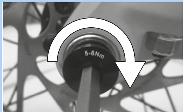
Figure 55: Tightening the securing screw
