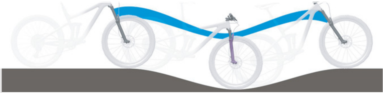
Figure 215: Excessively soft suspension in the suspension fork on hilly terrain
