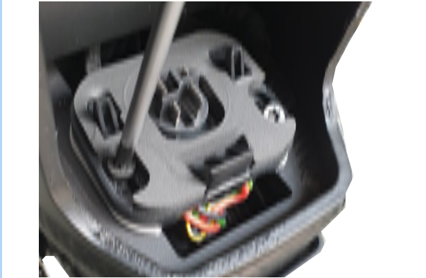
Figure 47: Undoing screws on battery mount
