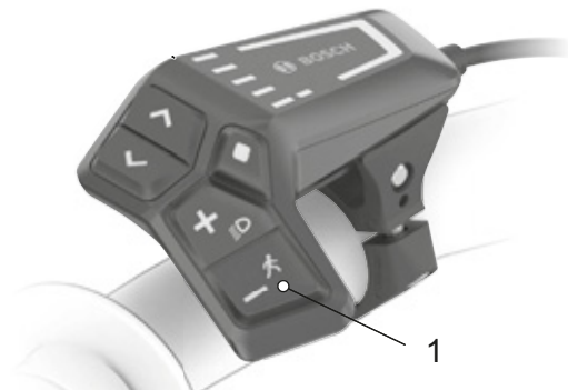
Figure 124: Position of push assist button (1)
