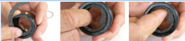
Figure 197: Inserting the felt ring
