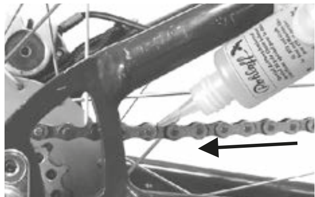
Figure 133: Lubricating the chain
