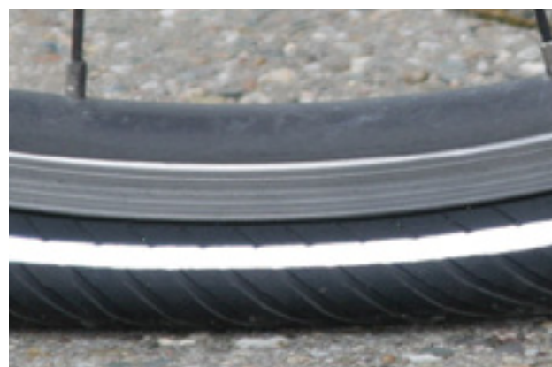
Figure 94: Much too little tyre pressure
