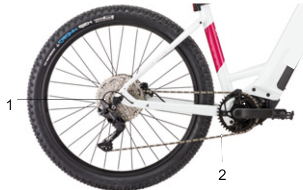
Figure 32: Chain drive with derailleur gears
