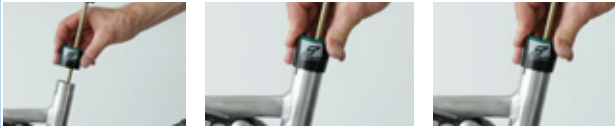
Figure 181: Attaching the outer sleeve
