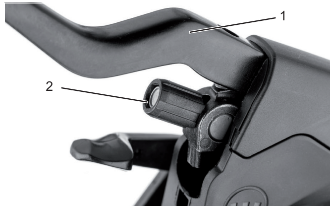
Figure 77: Brake lever (1) of the hydraulically operated rim brake with setting bolt (2)
