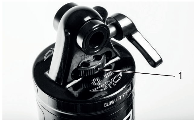
Figure 55: Suntour rebound adjuster wheel (1) on the rear frame damper
