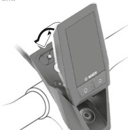
Figure 86: Folding the on-board computer.
