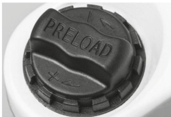
Figure 71: Negative deflection setting wheel on the suspension fork crown
