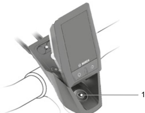
Figure 87: Position of headset screw
