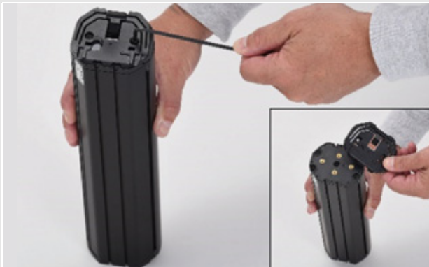
Figure 33: Detaching the upper interface
