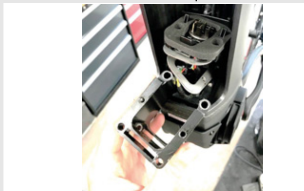
Figure 30: Pulling out the PowerTube adapter
