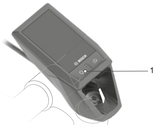
Figure 89: Position of On-Off button (on-board computer)
