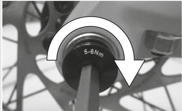
Figure 43: Tightening the securing screw
