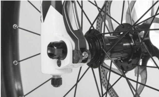
Figure 101: Adjusting the quick release clamping force
