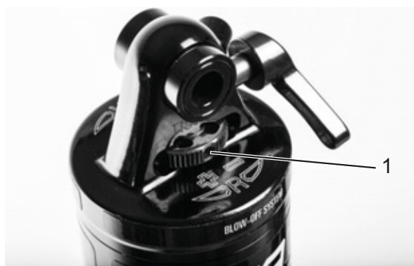
Figure 75: Suntour rebound adjuster wheel (1) on the rear frame damper
