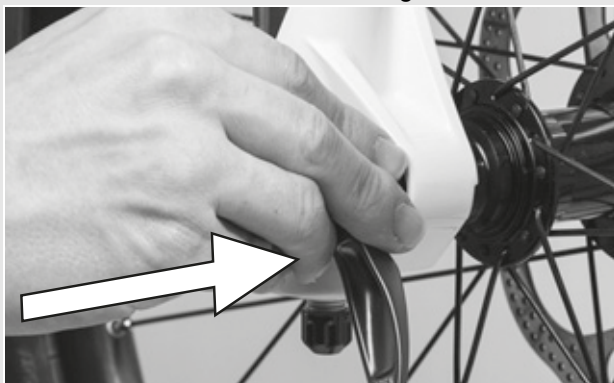
Figure 53: Pushing the quick release in
