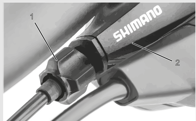
Figure 103: Adjusting sleeve (1) for the single-cable, cable-operated gear shift with shifter housing (2), example
