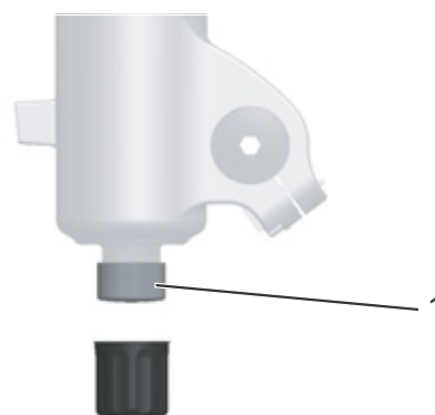
Figure 74: FOX rebound adjuster (1) on the fork end
