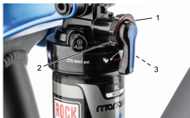
Figure 96: Setting the rebound damper strength on the rear frame damper setting wheel (1)
