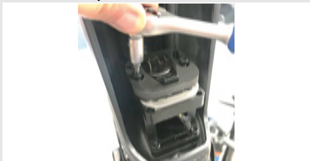
Figure 27: Undoing screws on battery mount
