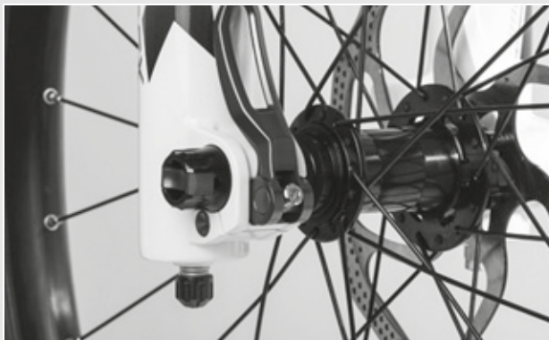
Figure 50: Perfect position for the clamping lever
