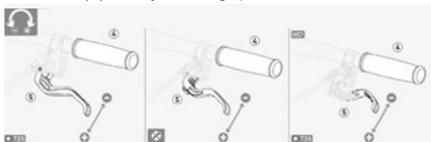
Figure 69: Setting the grip distance on a Magura disc brake lever
